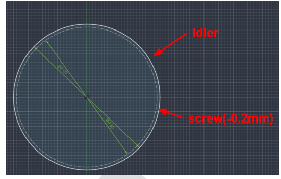
Fig. 3. An idler mounted on an M5 screw. The screw's shank is undersized relative to nominal, so the bearing bore is a clearance fit on it and the idler's axis can sit anywhere within that clearance.
