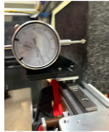
Fig. 11. Rail parallelism by dial indicator. The gauge rides the carriage and reads against a granite block clamped to the frame. The reference is the granite, never the extrusion.
