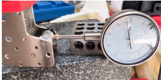
Fig. 10. Runout verification. The assembly is squared between granite blocks and a dial indicator reads the idler's running surface at several angular positions and at several heights. Disagreement between heights indicates the pin is not perpendicular.
