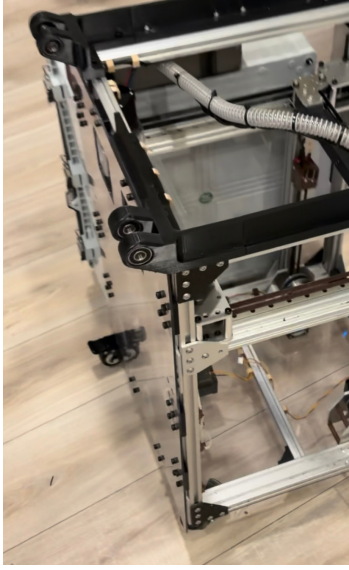
Fig. 1. Boaz in its final configuration: two-tier 20 × 40 mm gusset-joined frame, CoreXY motion on a carbon-fibre X beam, a three-actuator belted Z axis carrying a kinematically coupled ATP-5 tooling plate, and a folding polycarbonate enclosure.
