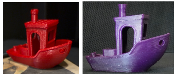
#SpeedBoatRace Benchies at the same 16 minutes: Boaz on the left, a Hev-Ort on the right. The smokestack is cleaner and the bow and stern carry fewer artifacts, both cooling-limited features, so credit goes to the duct and blower. One paired print is an anecdote, not a margin.
