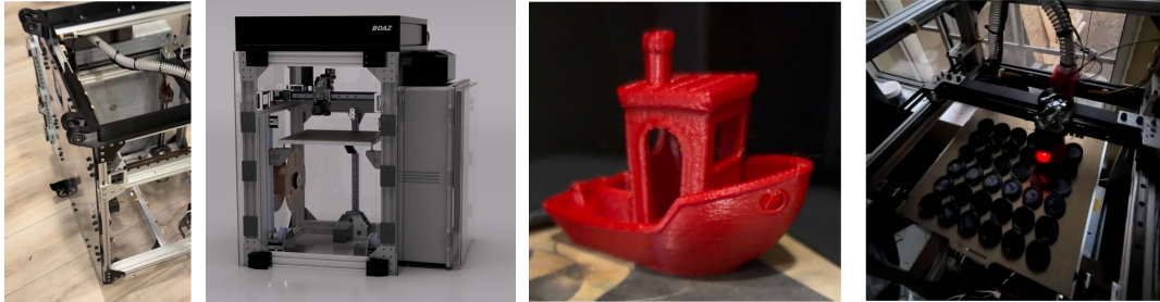
Boaz in its final configuration; the CAD assembly it was built from; a #SpeedBoatRace Benchy printed in 16 minutes; and plates of PETG medicine boxes from the production contract.
